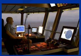
A bridge officer at the DP station, in constant communication with the ROV navigator
