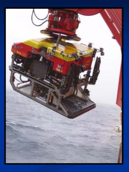
Step 3: Left: When Isis is underneath the gantry, the pilot turns parallel to the ship, and the winch lifts the vehicle out of the water. Good judgment is needed in rough seas to avoid the cable going slack, then snatching, as waves go by. Sterp 4: Right: Nearly home - Isis then latches firmly into the head of the gantry, to avoid swinging as it is brought on deck.
