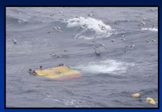
Step 1: Vehicle surfaces, staying away from the side of the ship, stern to, while the buoyancy floats are removed one-by-one.
