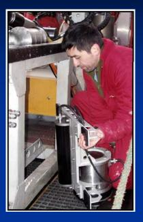
Installing the SM2000 echosounder to the under-frame of Isis. It uses a curved transducer to achieve a swath coverage of 60° either side of centre. Multiple beams are formed by control of phase.
