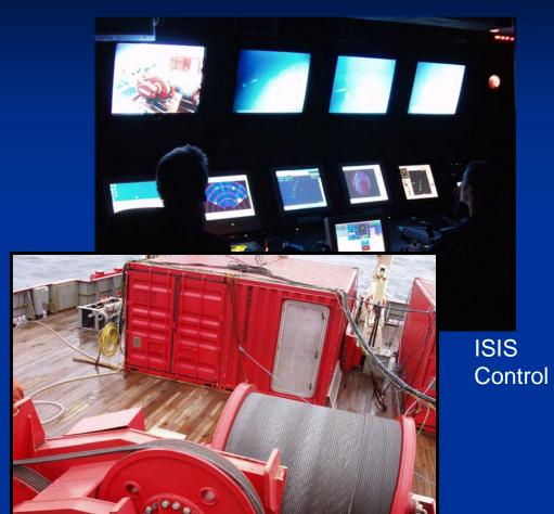
Winch and cable drum with 10km cable. Three optical fibres for data and three conductors at 3kV for power.
